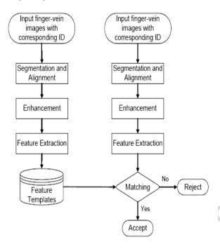
Fig.2.Arechitectural diagram of planned system
