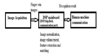
Fig.1.Haredware structure of a system
