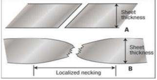
Figure: Fracture profiles of brittle fracture (A) with none through-thickness dilution, and ductile fracture (B) showing extensive localized dilution.
