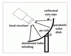
Fig 5 Parabolic solar dish collector
