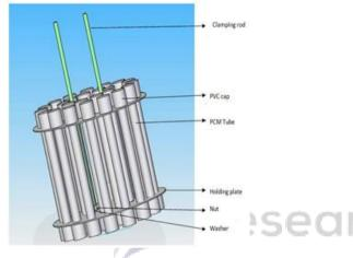
Fig. 6 Heat exchanger
