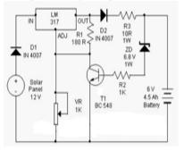
Considering the fig.4 represent the device controller circuit, within the controller circuit to controls the output voltage of the cell and furthermore on stop the battery from over voltage. Cell output voltage is oscillated attributable to climate changes thus we tend to area unit exploitation this charge controller circuit to stop the battery and once the battery return saturation region charge method is finished.
