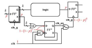
LACG takes AGFF a leap forward, addressing three goals; stopping the clock pulse also in the master latch, making it applicable for large and general designs and avoiding the tight timing constraints. LACG is based on using the XOR output in to generate clock enabling signals of other FFs in the system, whose data depend on that FF.
