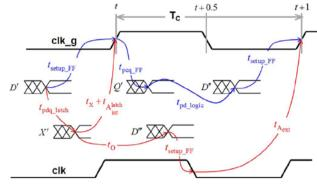
Using a FF for gating is a considerable overhead that will consume power of its own. This can significantly be reduced by gating FF'' Notice that since is oppositely clocked and its data is sampled at the clock's falling edge, its clock enabling signal must be negated. Also, is an ordinary FF where the internal XOR gate is connected between and D" and Q".
