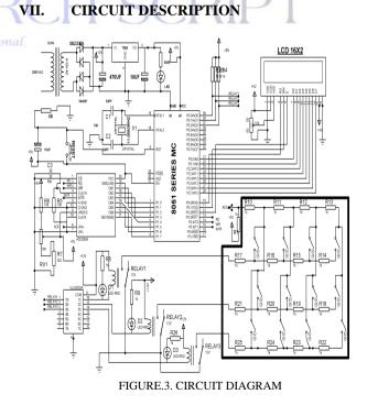
**1. Power Supply:** The circuit uses standard power supply comprising of a step-down transformer from 230Vto 12V and 4 diodes forming a bridge rectifier that delivers pulsating dc which is then filtered by an electrolytic
