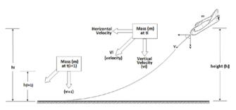
Fig. 3. Determination of landing path
