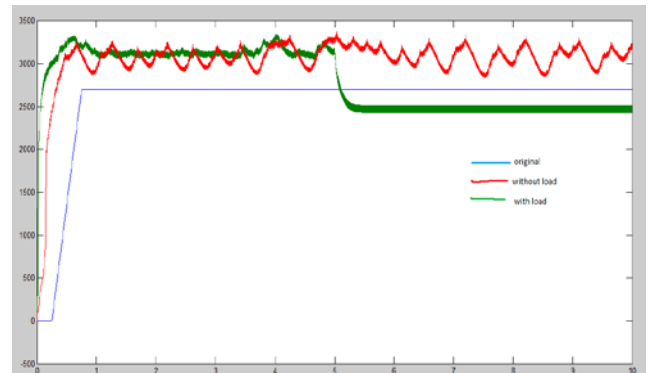
Fig 2: IM speed control by trail and error method with and without load
