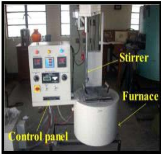
Figure 1 Stir casting Setup
