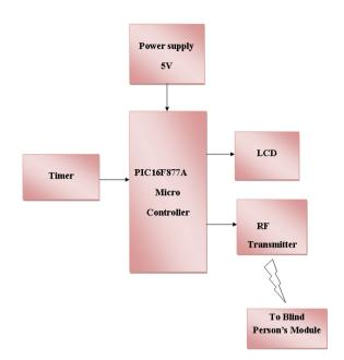
Fig. 2. Block Diagram of Traffic Module
