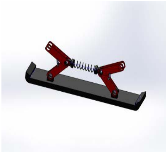
Fig. 1. This the Schematic diagram which shows how the shock absorber attached to the bumper with the help of arms and links.
