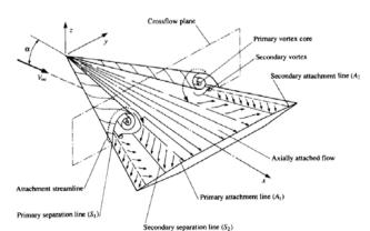
Figure 1: Flow over a Delta Wing at Incidence
