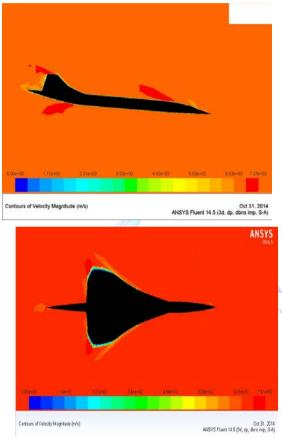
Figure 6: Side View and Top View of Velocity Countour
