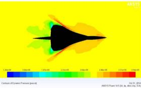
Figure 4 : Side View and Top View of Dynamic Pressure
