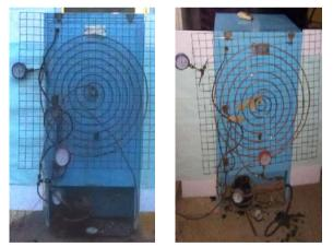
Fig.3.3 Spiralwith Pitch(38.1mm) Fig..3.4 Spiral with Pitch(44.45mm)
