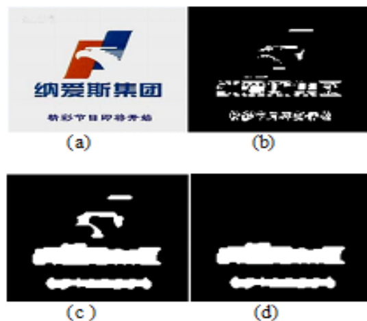
Fig.4 Candidate Text Region (a) Original Image (b) Candidate Text Pixel in First Scale (c) Horizontal Candidate region by Close Operation (d) Text region Detection by Density Based Region Growing
