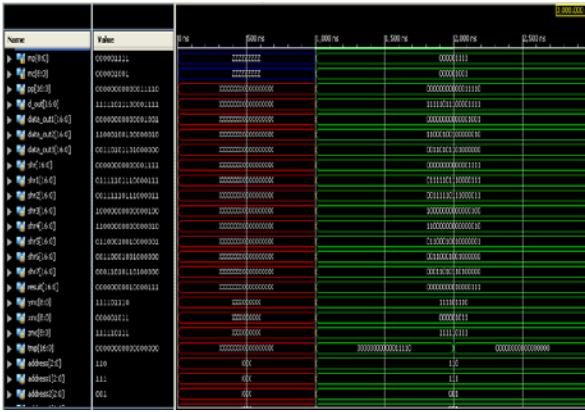
Fig 8 : Booth multiplication for Radix 4 Algorithm
