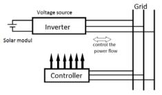
Fig.1 a: Basic Block Diagram of Gird Connected Inverter
