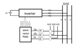
Fig.1 b: Basic Block Diagram of Gird Connected Inverter with PI controller
