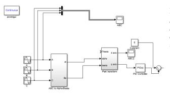
Fig. 2: Phase-Locked loop
