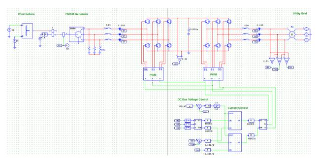
Fig.3.Simulation of Pwm Converters in PMSG in Wind Power System
