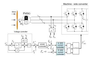
Form the Fig.2.circuit diagram
