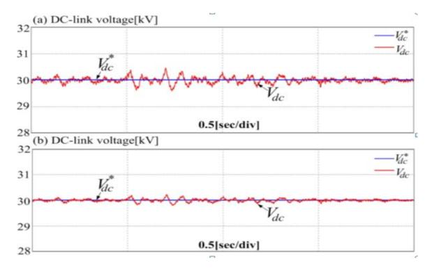
Fig.5. (a) and (b) Dc Link Bus Voltage Waveforms
