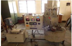
Fig.1. Stir casting setup
