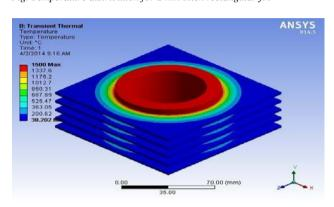
Fig. Temperature distribution for 3 mm thick rectangular fin
