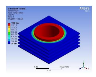
Fig. Temperature distribution for 2.5 mm thick rectangular fin
