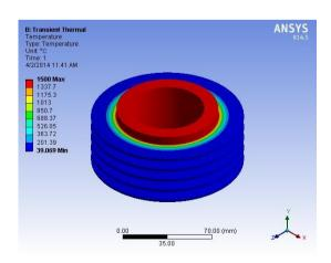
$Fig.\ Temperature\ distribution\ for\ 2mm\ thick\ circular\ fin$
