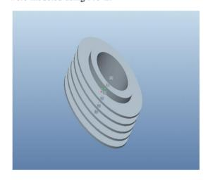
Fig.3 Circular cylinder fin
