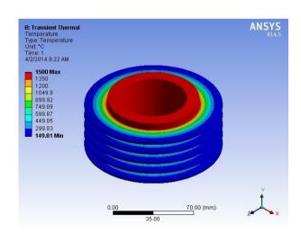
$Fig.\ Temperature\ distribution\ for\ 2.5\ mm\ thick\ circular\ fin$
