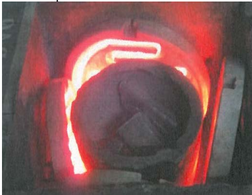
Fig 5: Crucible containing Al with heating coils
