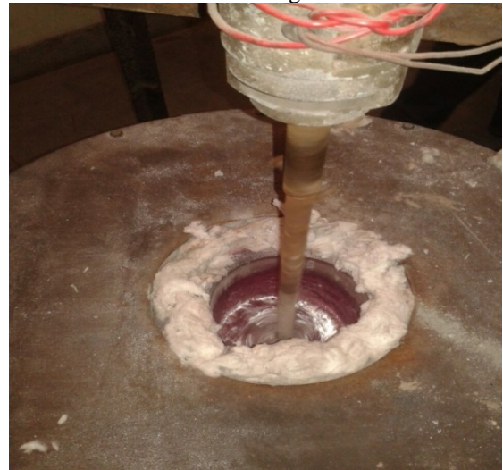
Fig8: Mixing of Fly ash in Molten Metal
