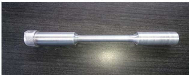
Fig11: specimen after machining
