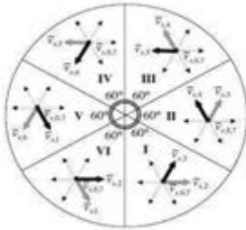
Figure 3 six equally sectors with different set of voltage vector
