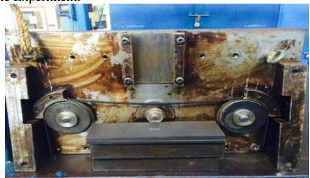
Figure 2 Preloading Setup – No Load Condition
