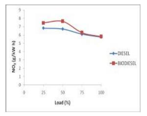
Fig.9 Nitrogen oxide Vs Load
