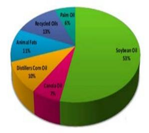
Fig.3 Various sources of biodiesel
