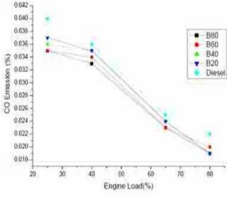
Fig.8 Carbon monoxide Vs Load
