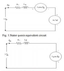
Fig. 2.Stator d-axis equivalent circuit
