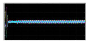
Fig 8. Three phase current with fuzzy controller
