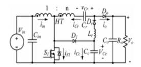
Fig.1 Proposed high step-up dc-dc converter with hybrid transformer
