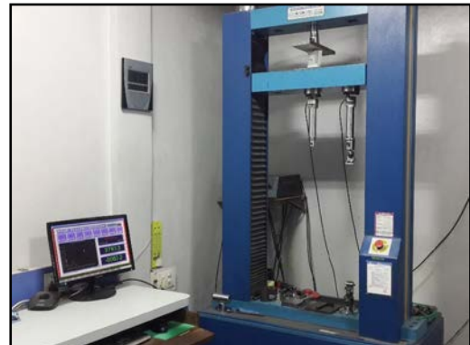
Fig. 1: Universal servo-electric test apparatus
