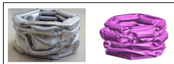
Fig 3 Deformed shapes of hexagonal crush cans obtained from testing and FEA
