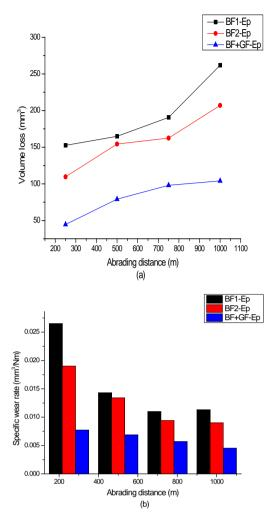
Figure 3: (a) volume loss V/s abrading distance and (b) Specific wear rate V/s abrading distance for different samples at 23N
