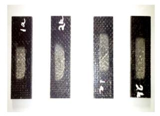
Figure 1: Three-body abrasive wear Specimens after testing
