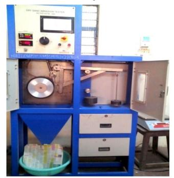
Figure 2: Three body abrasive wear setup
