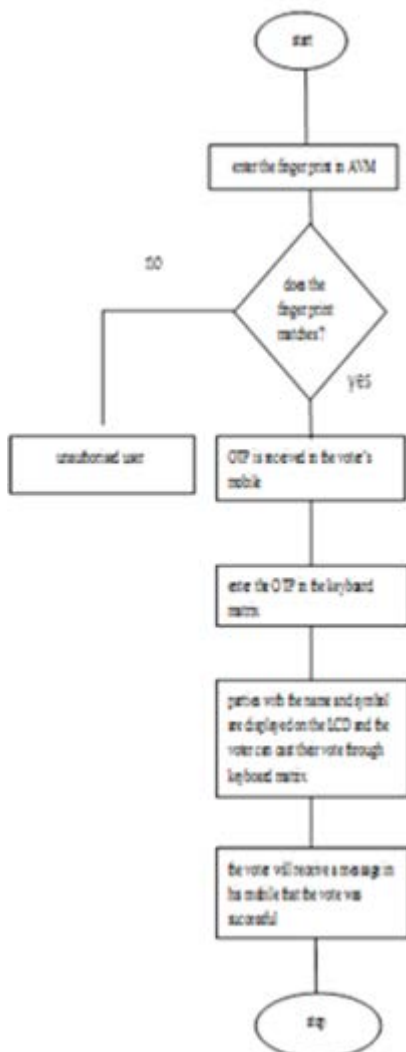
fig 4. Flow chart of smart voting system using AADHAR
