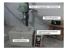
Fig. 1.Stir Casting Setup
