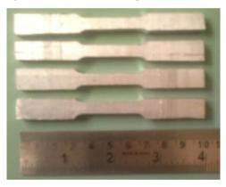
Figure 5: Tensile Test Specimen.
