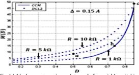
Fig-4.1 Ideal converter gain vs. duty cycle for variable switching frequency operation
