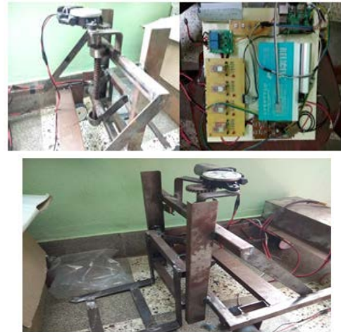
Fig 5: Pick and place robot with the electronic setup
