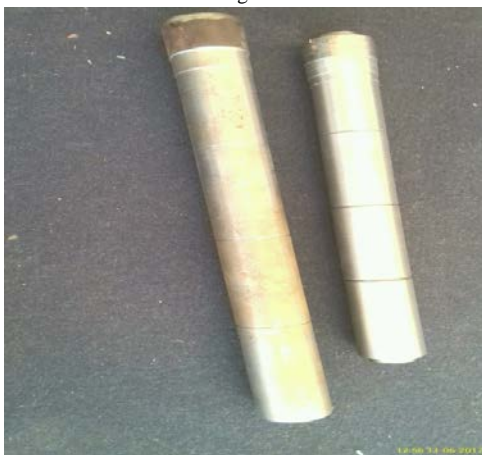
Figure 6.1: work piece EN 8 and stainless steel 305
