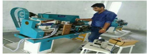
Figure 5.0: Working model of electromagnetic abrasive finishing
