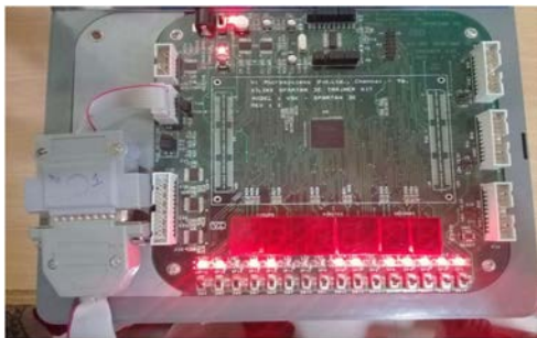
Fig. 14 Hardware Output of Dadda Multiplier
