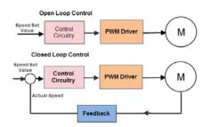
Fig.2.1. open and closed loop control
