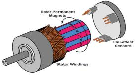
Fig.1.2 working of BLDC motor
