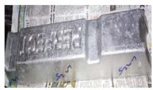
Figure 1 Aluminium lm25 ingot
