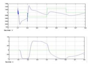
Fig 4.2.2 Measured Generator Power Output For Three-Phase Fault With E-Statcom
