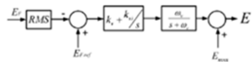
Fig 3.2 P V bus control topology for output voltage The synchronization and damping powers attenuate load angle and frequency fluctuations around equilibrium point and synchronize the VSC with the grid. Beside the inherent synchronization with the grid in steady-state,
