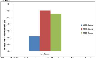
Figure 2. Effect of change in magnetic flux density on Magnetic abrasive machining
