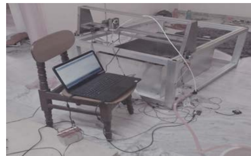
Fig 4: The picture depicts the working procedure of the system in which the whole functionality of the system is visualized and performed in action. The web module used by the user will give the instruction and the Wi-Fi module placed on the arduino will receive the signal and gives instruction to perform the actions and the Stepper motors, sensors, pumps and drivers will be operated based on the instruction provided by the microcontroller and this whole setup is powered by a single 12v battery charged using a 12v Ac to Dc converter.
