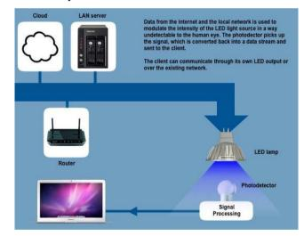
Fig. 1.1 Working principle of Li-Fi
