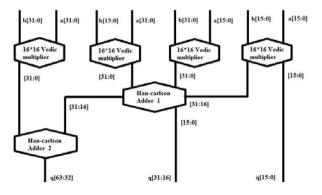
Fig.4.1 Block Diagram of proposed method using Han-Carlson
