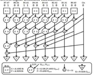
Fig.2.1 Block Diagram of Kogge Stone Adder.
