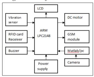
Fig 2: Block diagram of ATC.
