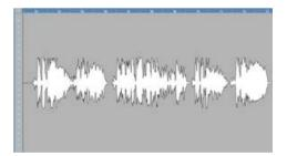
Here, the clipped flat ends will be finished as curves after compression. In other words, the clipped wave ends are compressed to a rounded wave peak. The mean or the average amplitude remains the same in both the recordings, but the peaks will differ. The amplitude range (difference between high and low amplitudes) will be very high before compression, but after compression the range will be minimized, making the signal sweet sounding
