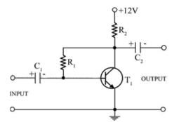
A Simplified Schematic of the Current-Sensitive Pre- Amplifier Circuit
