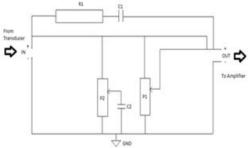
The potentiometer P1 is used to set the threshold level. Potentiometer P2 with the help of capacitor C2, changes the characteristics of the wave which is to be compressed. It must be mentioned that the compressor circuit does not require
