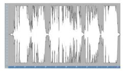
In the above simulation figure, it is the recording of a normal audio. We can observe that the peaks are ranging beyond the maximum limit. Hence the peaks of the waves are clipped. Clipping results in a loss of information such high scale audio. The below simulation is the same audio recorded through the microphone designed in this project.
