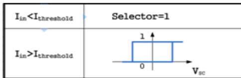
Figure 7 Logic decision of super capacitor converter
