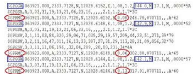
Fig. 10. Experimental result of GPS information with GGA (blue) and RMC (red) parameters.
