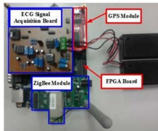
Fig. 4. Multi-function H-Box with FPGAVB multi-modules
