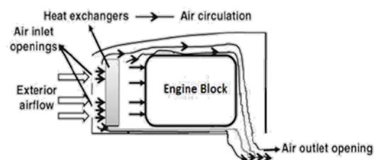
Figure 1: Schematic of the complex air flow through the under hood compartment.
