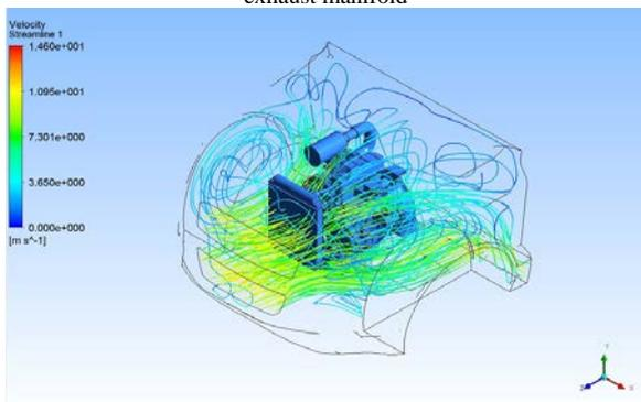
Figure 6 Streamlines launched from the domain inlet, drawn over the plane passing through the radiator, engine, exhaust manifold and the brake booster.
