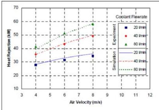
Figure 3 Heat exchanger performance data.
