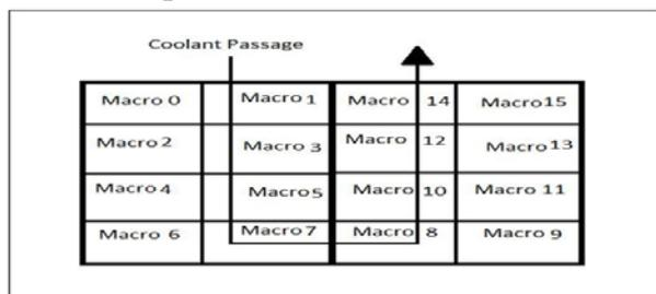
Figure 2: Heat exchanger core divided into  $2 \times 4 \times 2$  macros
