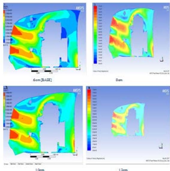
Figure 4: Contours of velocity on a plane through the engine and the exhaust manifold.
