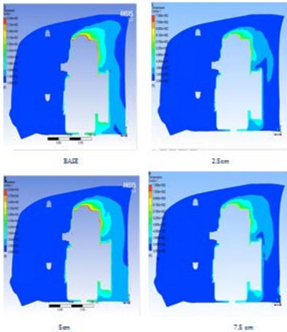
Figure 5: Contours of temperature on a plane through the engine and the exhaust manifold
