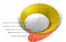
However, it is equally important to consider particle size and the fluid cleanliness level required for journal bearing operation. Removal of clearance-sized particles is required for wear reduction and scuffing failure, and can be achieved by implementing high efficiency filtration to lubrication systems equipped with journal bearings.
