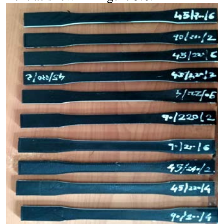
Figure 3.2 ASTM D638 specimens
