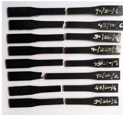
FIGURE 3.3 ASTM D638 specimens after testing
